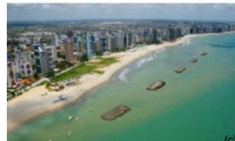
Hard protective structures for coastal management: (a) Seawall in Isle of Wight (Source: Oikos-team, 2007); (b) Groynes in Sitges, Catalonia, Spain (Source: Jordi Serra, 2007); (c) Detached breakwaters in Brazil (Source: UFPE); (d) Beach nourishment in Hayling Island, England (Source: ESCP); (e) Accommodation & Advance responses (IPCC, 2019)
